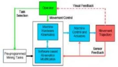
Fig.2. Functional Block Diagram of the New Robot Human Control Architecture
