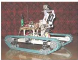
Fig. 5 The complete robot unit with the pan-and-tilt mechanism for better navigation
